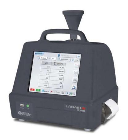
The Lasair III particle counter sets the new standard for aerosol particle counters. The on-board Pulse Height Analyzer (PHA) ensures ISO 21501 compliance. The large IR touch screen controls and intuitive user interface make the system very easy to use. The particle counter's rugged enclosure is chemically resistant and lightweight for portability. The enclosure also has a streamlined design that minimizes particle traps and makes the unit easy to clean.
